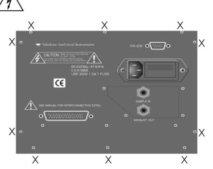
Figure 5-4: Rear Panel Removal (Remove only those screws marked with an X)
